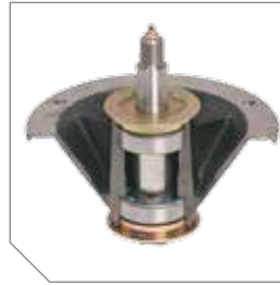
Cast-Iron Spindles longer usable life, 25,4 mm shaft with top access grease fitting for greaseable dual ball bearings, six-bolt 203 mm flange design adds strength and greater dispersal of energy to deck assembly.
